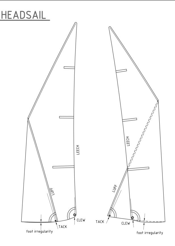
The foot irregularity is defined as the maximum distance between the edges of the foot when first the lowest point of the luff and then the lowest point of the leech are superimposed on any part of the foot.
